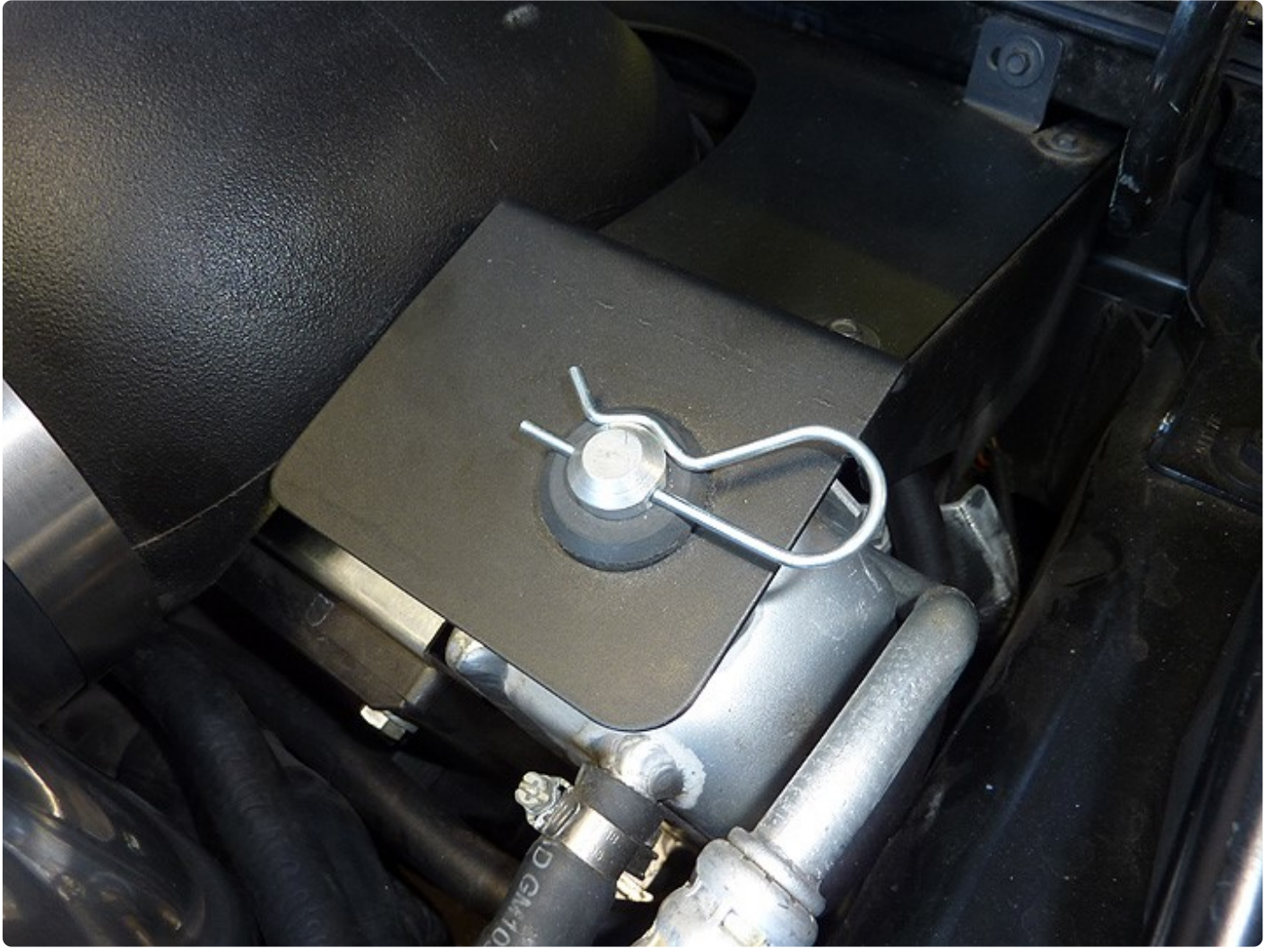
(LEFT AND RIGHT COTTER PINS INSTALLED)
