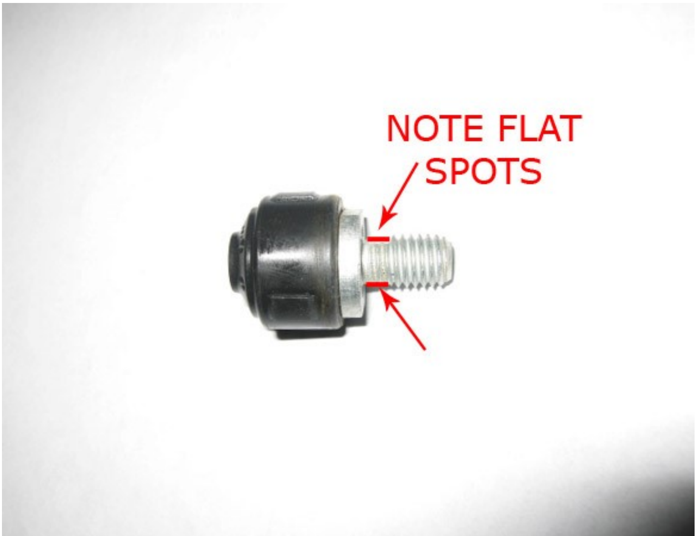
(ABS MODULE MOUNTING STUD)
