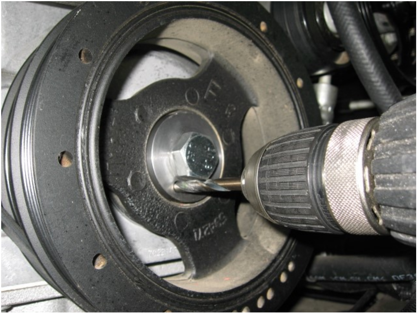
(DRILLING CRANK AND BALANCER THROUGH PIN FIXTURE)
