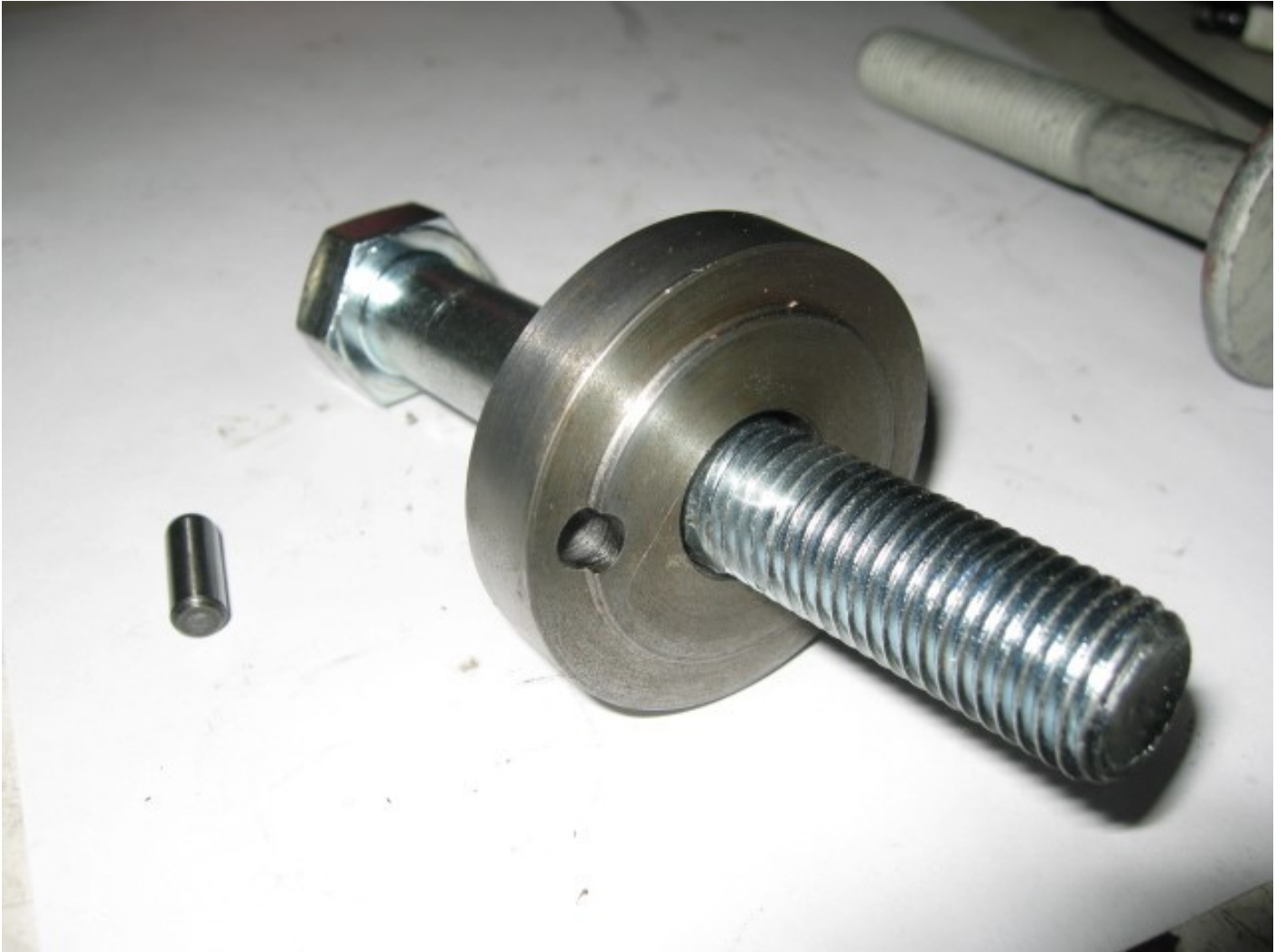
(PIN FIXTURE WITH BOLT AND PIN)
