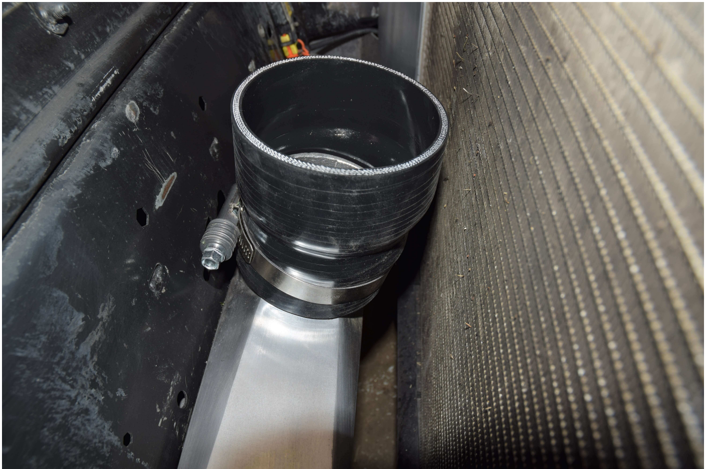
(ANGLED COUPLER BETWEEN INTERCOOLER AND MAF TUBE)
