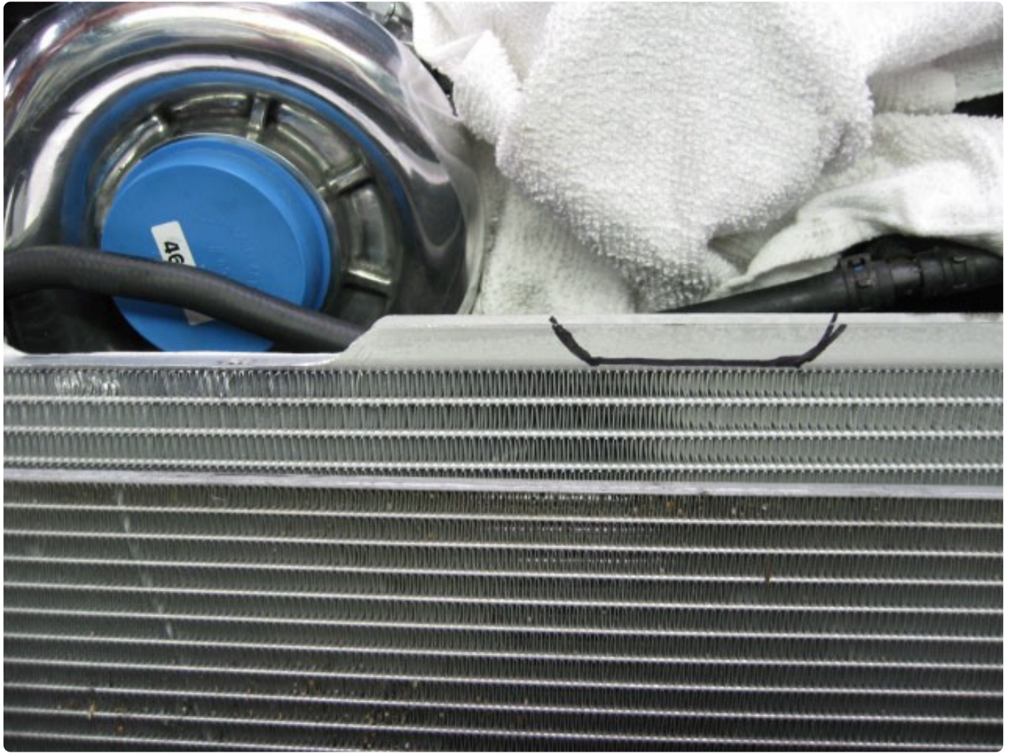
(RADIATOR MARKED FOR TRIMMING)
