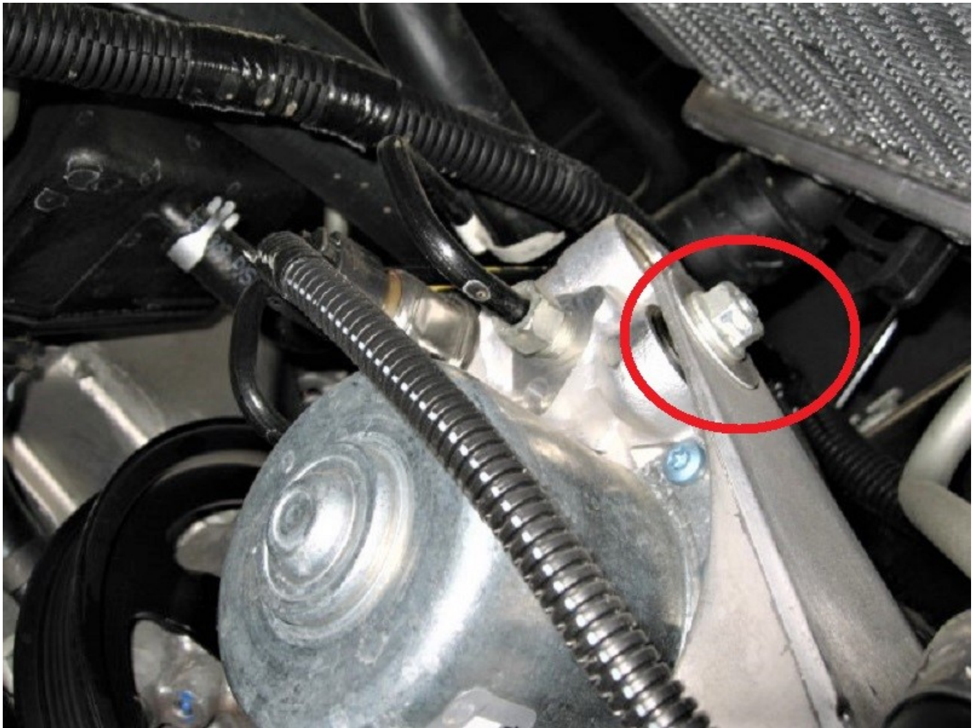
(ABS MODULE – MOUNTING STUDS)
